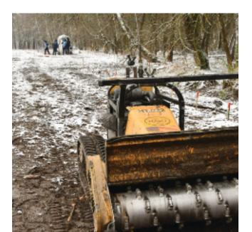
HALO is already investing in both technological innovation and innovations in process to ensure it has the right mix of techniques for the huge task ahead. Armoured, remote-controlled mechanised clearance will be a part of the mix. Drones carrying sensors, such as lidar and thermal cameras, will help with mine detection.
